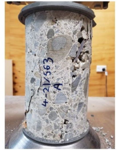
Figure 1: Core sample 4-21/563A before and after testing.
