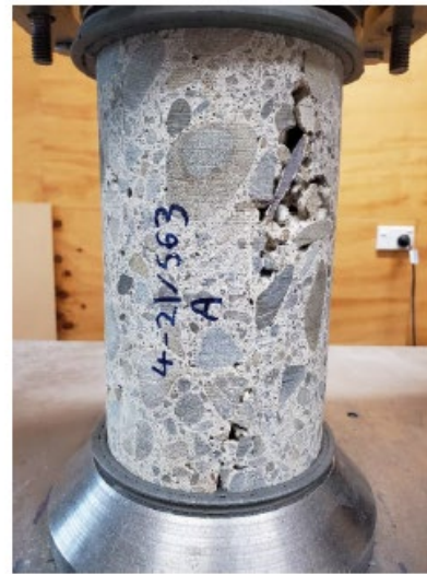
Figure 1: Core sample 4-21/563A before and after testing.
