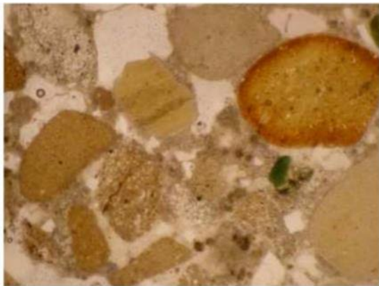
Figure 1: Photomicrograph, typical field of view of concrete from interior of Gisborne Cenotaph, showing fine aggregate particles of calcareous and other mudstone set in limey paste (higher relief, pale grey). Note oxidised rim to clast at top left. Colourless areas have lost friable paste during specimen preparation. Transmitted light. Scale: width of view is 6 mm.
