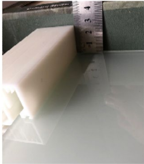
Re-designed, reduced height (reduced by 8mm in total when gasket in place)
